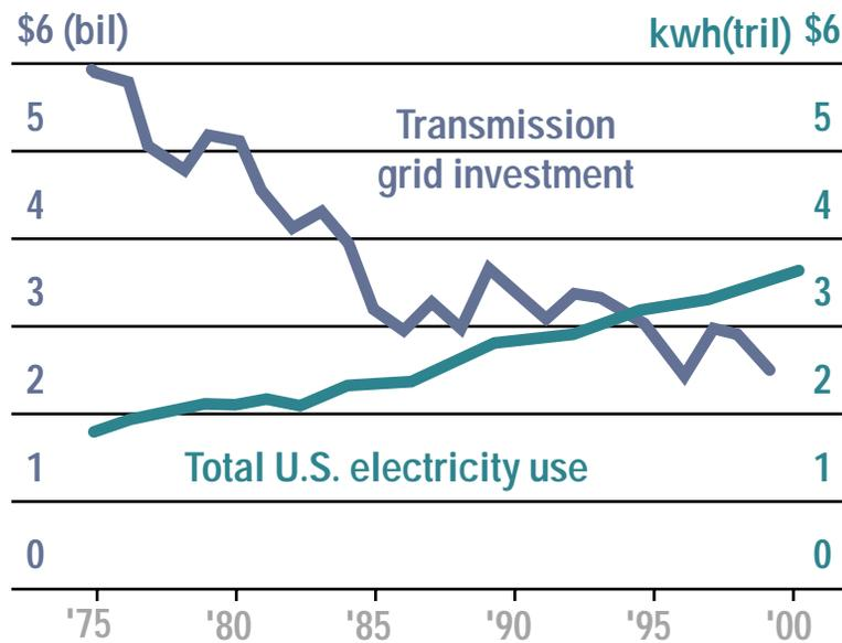
Figure 1. Transmission grid investment vs. energy consumption. Source: Edison Electric Institute; U.S. Department of Energy.
